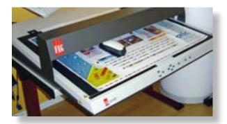
Colorimetric devices are available as spectroscopic or as combined instruments (density plus spectroscopy), and also available either as hand-held instruments or as scanning spectroscopes (FAG Spectromat).
