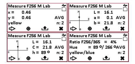
Bi-Fluorescent Analysis is available only in F256 Mode. Any measurement in F256 Mode is based on two readings, one with UV 256nm illumination and the second one with 365nm illumination. The Bi-Fluorescent Analysis screen shows the following values:
