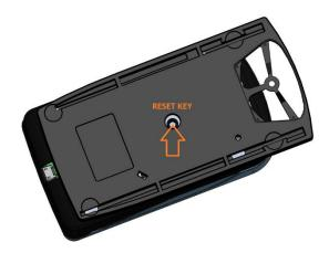
After a Hardware Reset the FLUO DX will show the key information about the device such as Serial Number, Device ID and Firmware version. Next to the Firmware version a character displayes the internal calibration version currently in use:
