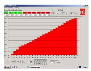
The image is captured by a high resolution CCD Camera. The ink key profile of the currently used printing plate is calculated within a few seconds using picture process algorithms.
