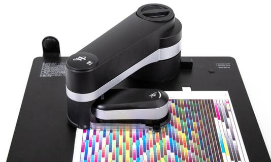
**i1i0** The optional X-Rite i1i0 automated chart reader captures hands-free measurements on printer profile charts. i1i0 accommodates both i1Pro 3 and i1Pro 3 Plus devices to enhance functionality and speed up the measurement process.
